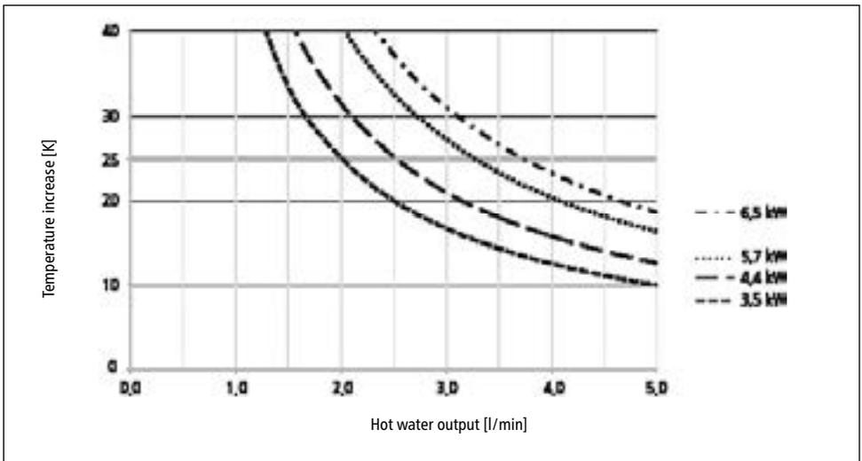
Fig. 12 "Temperature increase and hot water output"
