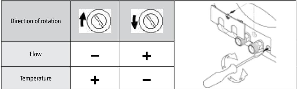
Fig. 11 "Adjusting the water flow and temperature"
